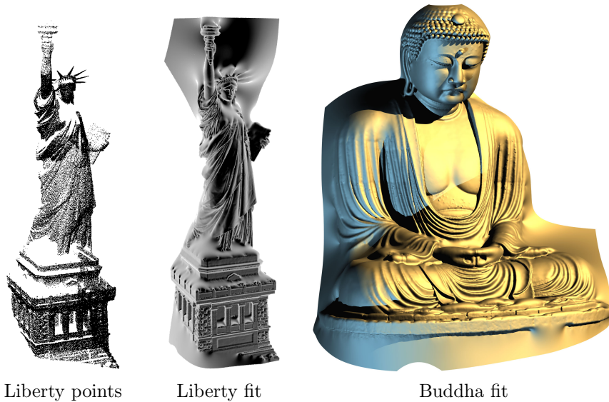
Fig. 1. LIDAR scans and smoothest restricted range reconstruction of the Statue of Liberty and a Buddha statue.
